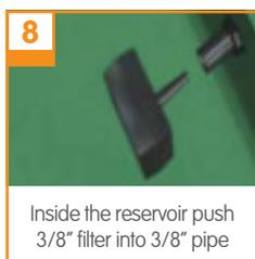
Inside the reservoir push 3/8" filter into 3/8" pipe
