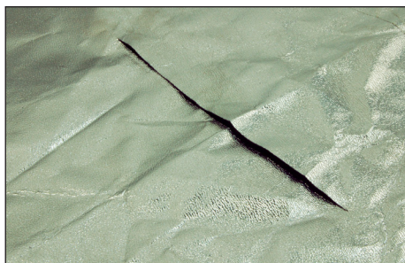
STEP 2: Locate the rip or tear on the inside of the grow tent skin. (Silver Side)
